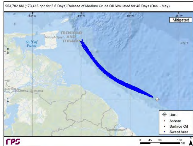
Mitigated – Uaru Project Wellhead 953,782 bbl (173,415 bpd WCD) Medium Crude Release – Season 2 (December – May)
