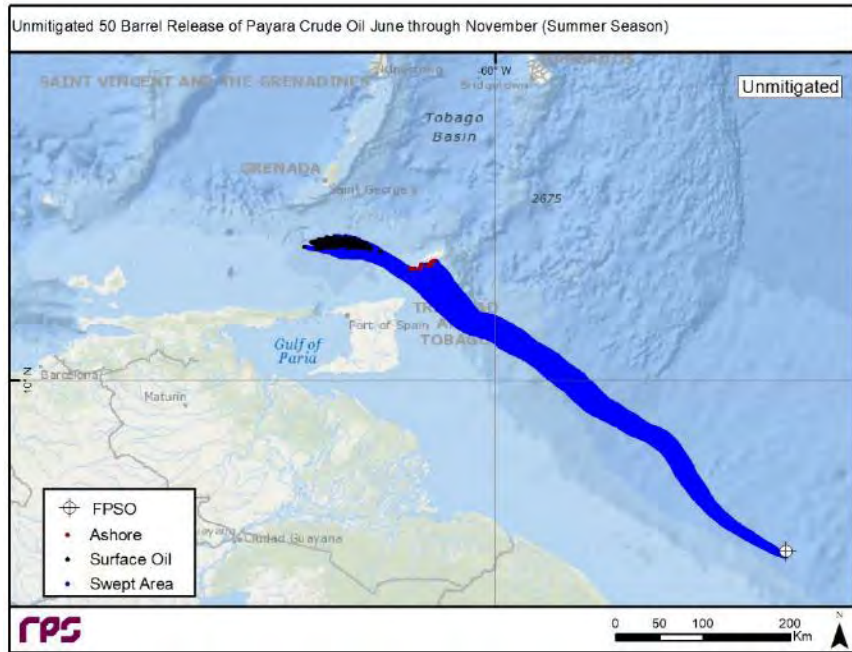
Figure B-15: Unmitigated area swept results for the 95th percentile minimum time to shoreline 50 bbl Crude Oil release during June through November season. Area swept is displayed in dark blue, surface oil droplets remaining at the end of the 10-day scenario are presented in black, and shoreline oiling is displayed in red.
