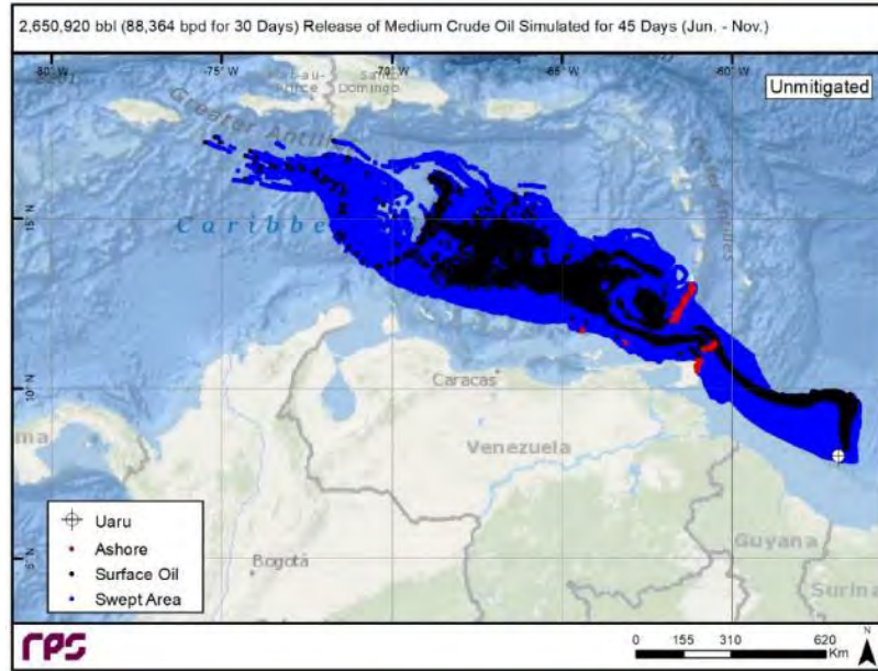
Figure B-41: Area swept by surface oil throughout 45-day model simulation for a 95th percentile minimum time to shore scenario for a 2,650,920 bbl (88,364 bpd Most Credible WCD) spill of medium crude at the Uaru Project wellhead during Season 1. Blue area represents surface area swept. Black points represent surface oil remaining at the end of the simulation. Red points represent shoreline oil remaining at the end of the simulation.
