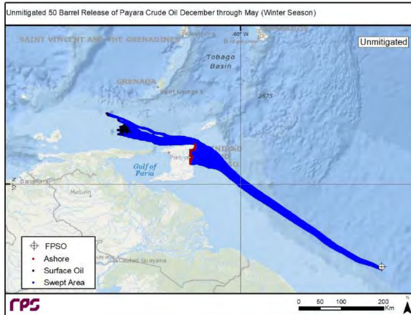
Figure B-18: Unmitigated area swept results for the 95th percentile minimum time to shoreline 50 bbl Crude Oil release during December through May season. Area swept is displayed in dark blue, surface oil droplets remaining at the end of the 10-day scenario are presented in black, and shoreline oiling is displayed in red.
