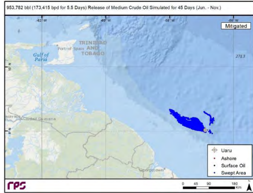
Figure B-46: Area swept results for the mitigated 95 th percentile time to shore scenario for the 173,415 bpd WCD release of a medium crude oil at the Uaru Project wellhead during Season 1. Blue area represents surface area swept. Black points represent surface oil remaining at the end of the simulation. Red points represent shoreline oil remaining at the end of the simulation.
