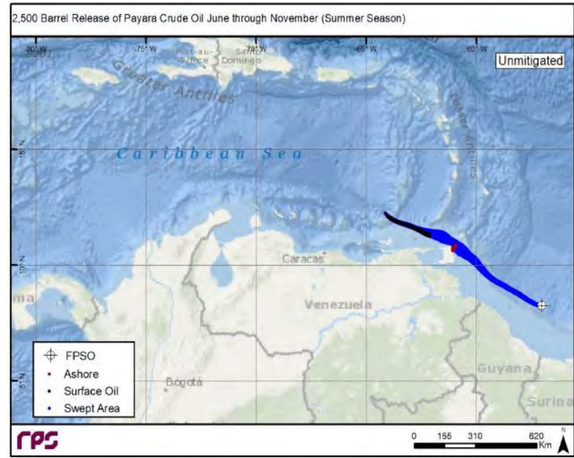
Figure B-16: Unmitigated area swept results for the 95th percentile minimum time to shoreline 2,500 bbl Crude Oil release during June through November season. Area swept is displayed in dark blue, surface oil droplets remaining at the end of the 10-day scenario are presented in black, and shoreline oiling is displayed in red.
