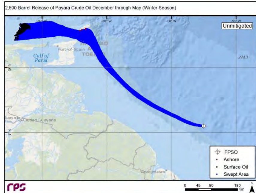
Figure B-19: Unmitigated area swept results for the 95th percentile minimum time to shoreline 2,500 bbl Crude Oil release during December through May season. Area swept is displayed in dark blue, surface oil droplets remaining at the end of the 10-day scenario are presented in black, and shoreline oiling is displayed in red.
