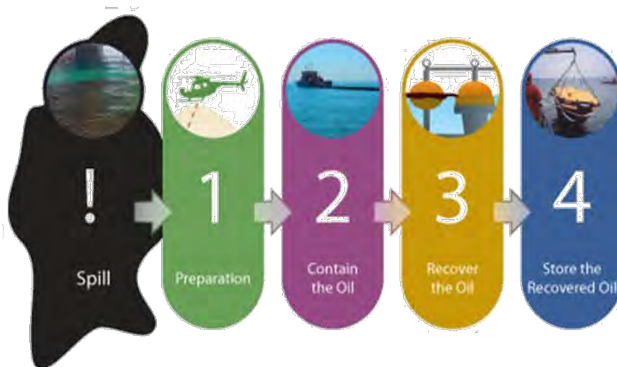
Figure 5-4: Harbour Containment and Recovery Key Steps
