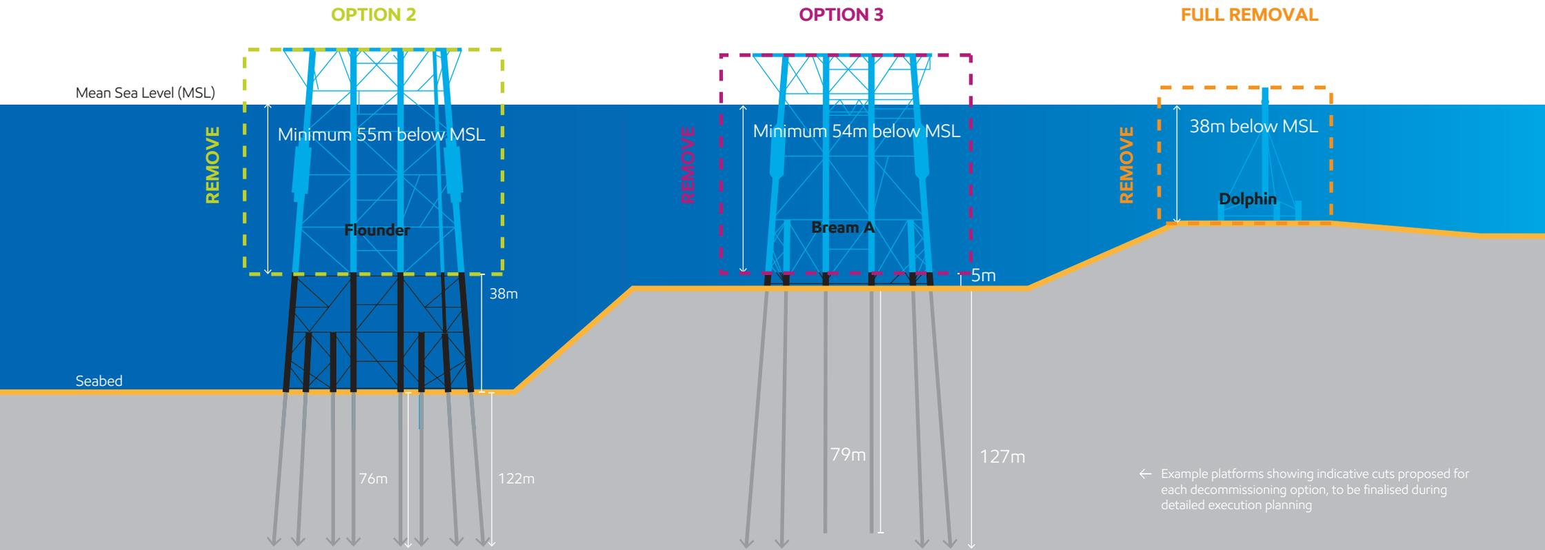
← Example platforms showing indicative cuts proposed for each decommissioning option, to be finalised during detailed execution planning
